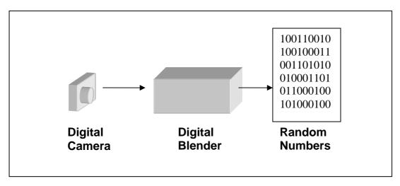
The digital blender is the most complex part of lavarnd. It consists of several types of data transformation operators to get as good random numbers as possible out of the physical process.
